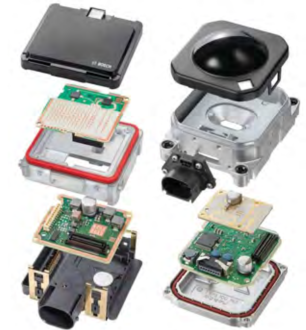
Construction of the Bosch RADAR sensors MRR and LRR3 (Source: Bosch)
