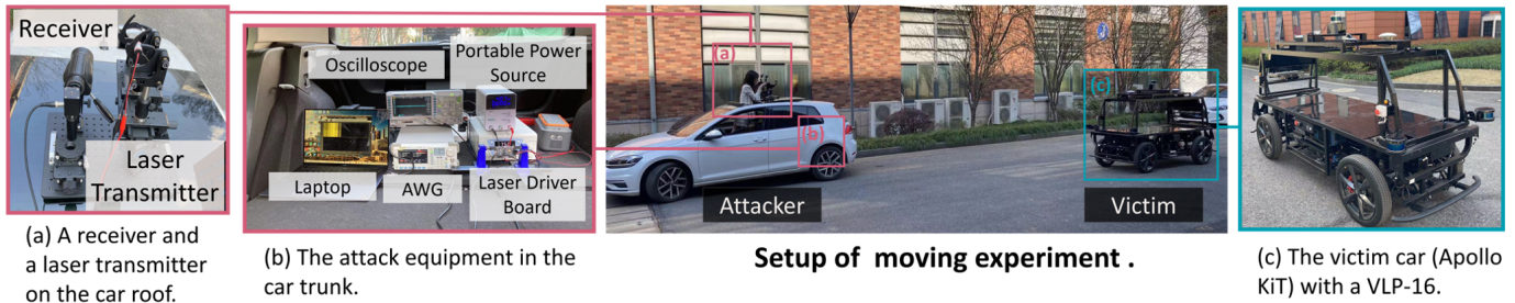
Fig. 19: Experimental setup for physical attacks on moving vehicles.
