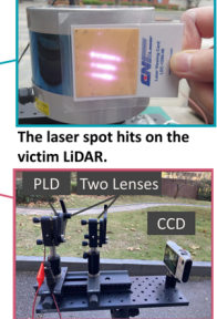
(b) Physical experiment setup consisted of a receiver, an arbitrary signal generator, a laser transmitter, and a victim LiDAR.
