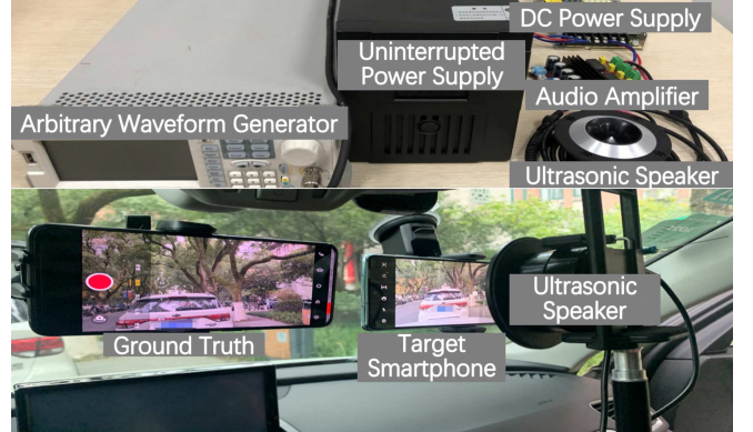
Figure 8: Experimental setups. An ultrasonic speaker beams designed acoustic signals to the target smartphone in a moving vehicle to launch PG attacks.
