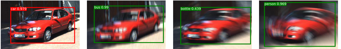
(a) Car detected without any motion blur (confidence score 0.979) (b) Car is misclassified as bus (0.99) after linear motion blur (slight, vertical) (c) Car is misclassified as bottle (0.439) after rotational motion blur (slight, anticlockwise) (d) Car is misclassified as person (0.969) after rotational motion blur (heavy, anticlockwise)
