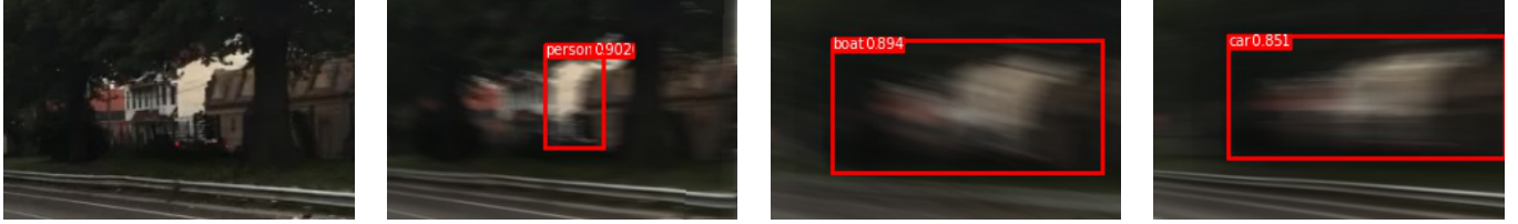
(a) Nothing detected for the original image without any motion blur (b) Person detected (0.902) after linear motion blur (slight, horizontal) (c) Boat detected (0.894) after linear motion blur (heavy, inclined) (d) Car detected (0.851) after linear motion blur (heavy, horizontal)
