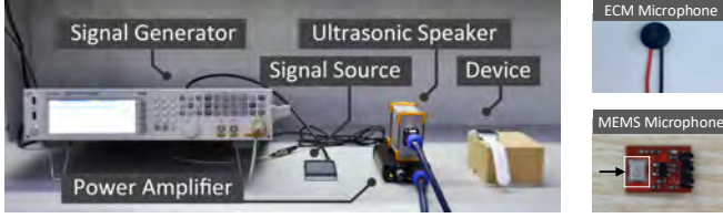
Fig. 4: An illustration of the benchtop experimental setup for investigating the feasibility of receiving ultrasounds with ECM and MEMS microphones. This benchtop setup is used for validating the feasibility of attacking various voice assistants as well.
