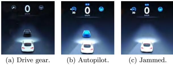
**Figure 9: Tesla dashboard display at drive gear, Autopilot, and Autopilot with radar jamming.**
