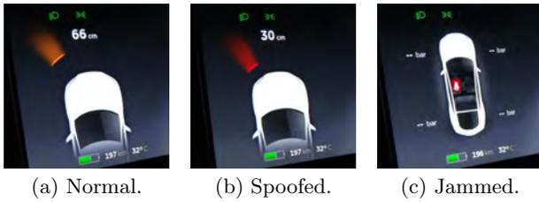
Figure 4: Tesla parking distance display at normal, being spoofed, and being jammed<sup>2</sup>.
